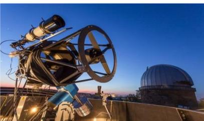
Uhlandshöhe Research Observatory, Stuttgart's first SLR station, using a fibre transmitter and a 100 kHz ranging laser.
