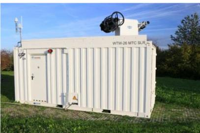
STAR-C, Stuttgart's new container-based space debris laser ranging platform currently under development.
